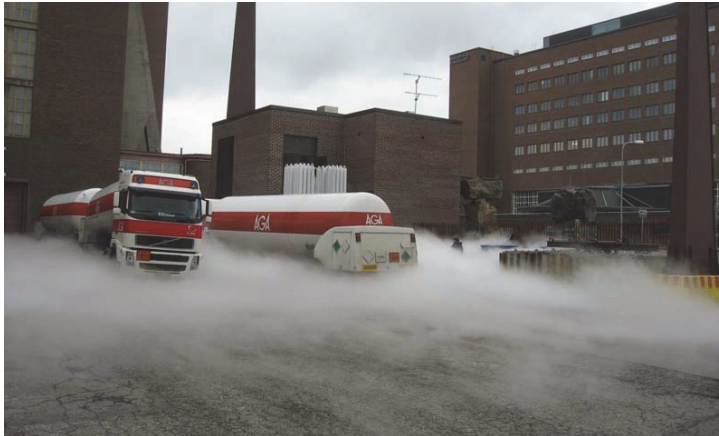
Figure 8. Nitrogen injection at the Salmisaari plant during the worst fire incident in 2008. Photo: Juha Sipilä/Helsingin Energia
