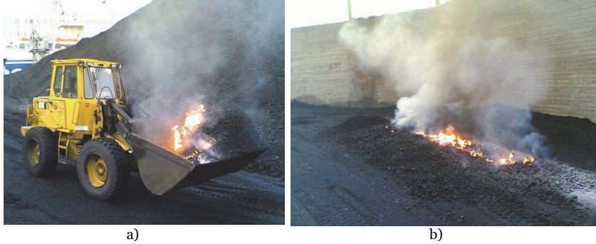
Figure 3. a) Excavation and removal of burning hot spot in an open coal stockpile; b) spreading out burning coal for self-extinction. Photos: Keijo Kotirinta/Helsingin Energia
