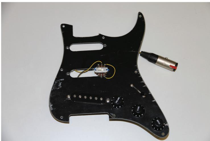
**Figure 5.2.** Pickup measurement setup used in Publication II.
