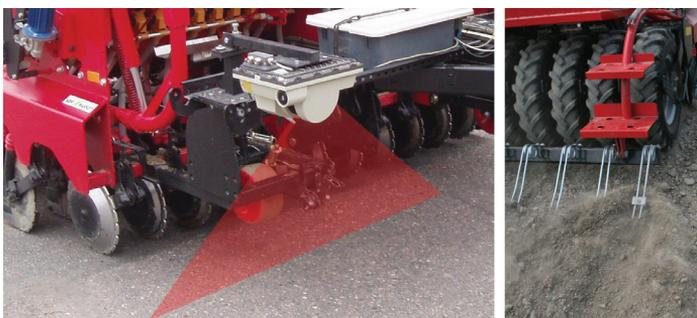
Figure 3.5. A laser scanner measured the profile of the ground (left). A furrow was produced at the edge of the sown area by a small plough, which was mounted on the following harrow of the seed drill (right).
