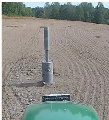
Figure 5.14. Test obstacle in front of the tractor.
