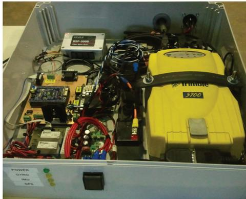
Figure 3.4. In measurement system II, the position and orientation of the tractor was measured with a Real Time Kinematic GPS, a Fibre Optic Gyro and an Inertial Measurement Unit, which were packed together.
