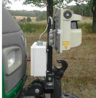
Figure 3.6. A laser scanner was used to detect the obstacles in front of the tractor.
