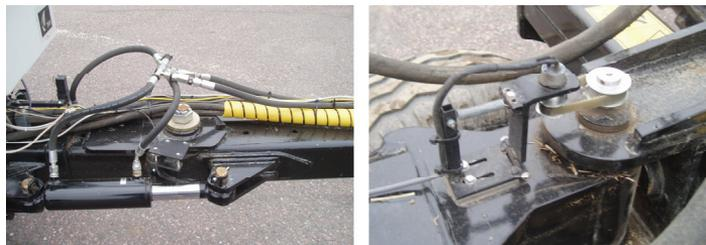
Figure 3.3. The articulated joint at the end of the drawbar (left), and the measurement of the freely moving joint (right).
