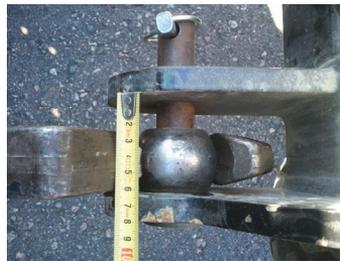
Figure 6.1. The mounting of the implement allows the implement to move a few centimetres sideways.
