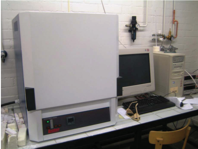
Figure 5. The equilibration experimental setup for the binary systems: a Lenton UAF 16/10 chamber furnace, S-type thermocouple, Keithley 2000 DMM, mercury thermometer and a PC for data logging.
