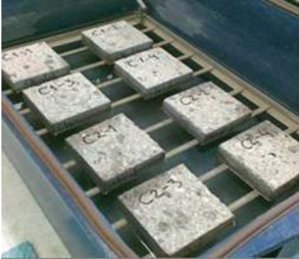
Figure 25. General arrangement of the capillary suction test.
