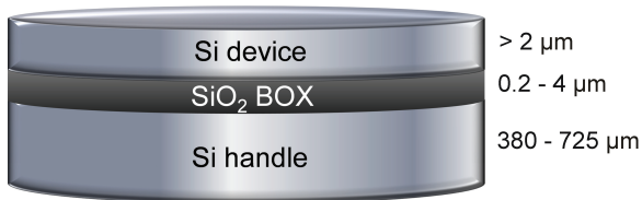
Figure 2.2. Silicon-on-insulator wafer structure. The dimensions are typical for bonded SOI wafers used in MEMS applications [27].
