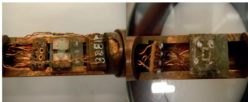
Figure 5 Close-ups of the Seebeck coefficient (left) and resistivity (right) measurement probes.
