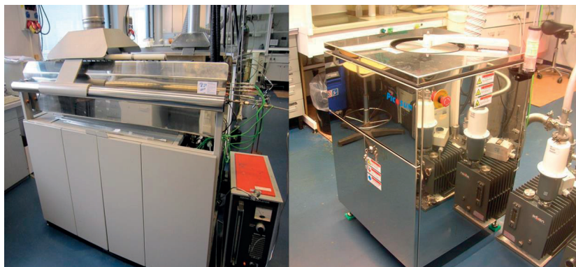
Figure 2 The two ALD reactors used in this study: the F-120 reactor on the left and the R-100 reactor on the right.
