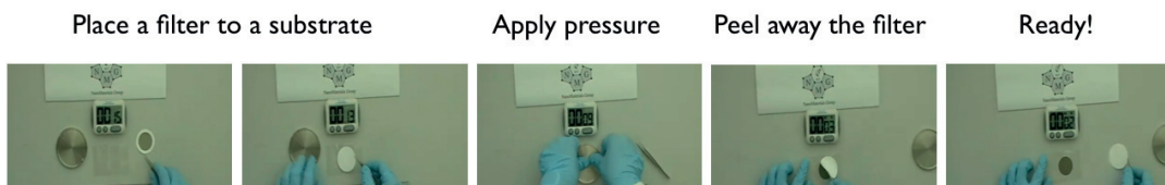
Figure 5.10. A typical manually performed room-temperature press transfer process. A filter with aerosol-CVD synthesised SWCNT network was placed on a substrate material, which was in this case a transparent PET-film. The SWCNT-network and the substrate were pressed together with moderate pressure around 1 kPa, by using a flat metal disk at room-temperature. Following this, the membrane filter was peeled of and the SWCNT films stays adhered to the substrate (Publication 1).
