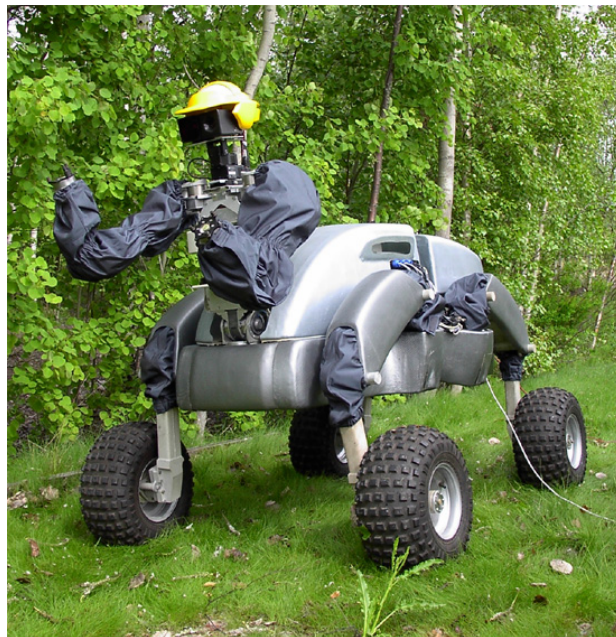
Figure 2.5. WorkPartner, mobile centaur-like service robot
