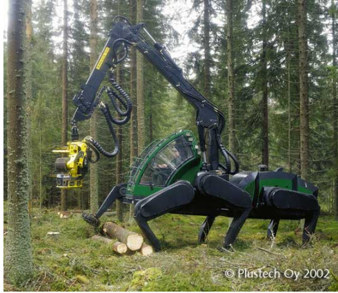
Figure 2.4. Six-legged Walking Harvester of Plustech. Courtesy of Plustech Oy
