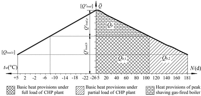
**Figure 2.2.** Heat load duration curve for a combined district heating system. The expressions in square brackets denote the relative position of the starting heat load and design heat load for the combined district heating system:  $t_w$ —outdoor temperature;  $N$ —cumulative heating time;  $\bar{Q}$ —relative heat load factor. Cumulative heat provisions for producing domestic hot water are excluded from the analysis.
