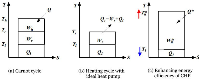
**Figure 3.5.** Ideal thermodynamic cycles and fundamental way to enhance the energy efficiency of CHP (Zhou & Hu, 2001).
