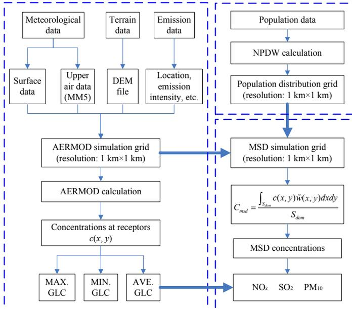
**Figure 3.3.** An overview of the AERMOD modeling and MSD calculation for NO<sub>x</sub>, SO<sub>2</sub>, and PM<sub>10</sub>.
