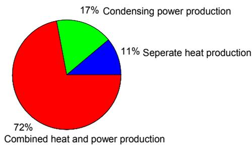
**Figure 1.5.** Fuel use by production mode in electricity and heat production 2011 (Statistics Finland, 2012).
