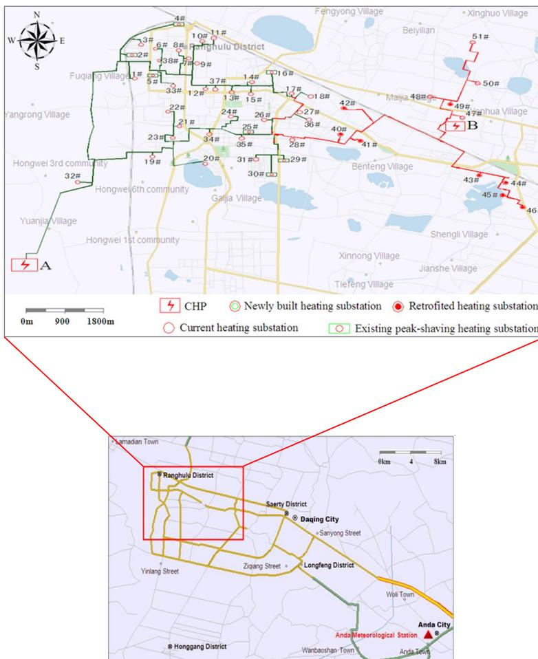
**Figure 4.6.** The position and topology of Daqing’s combined district heating system. Anda Meteorological Station is also labeled at the bottom using a solid triangle.
