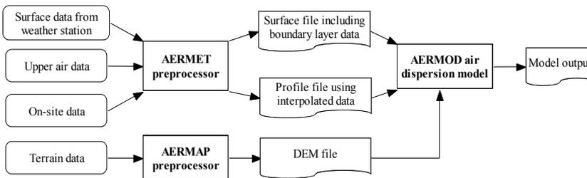
**Figure 3.2.** Structure of AERMOD model system.
