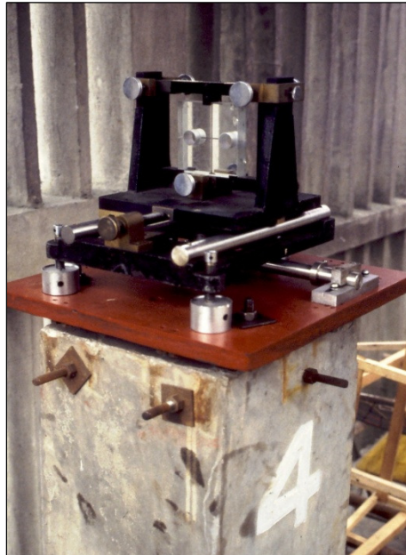
Figure 5.12 Mirror equipment on pillar no. 4 (at 6 m in interference observations).
