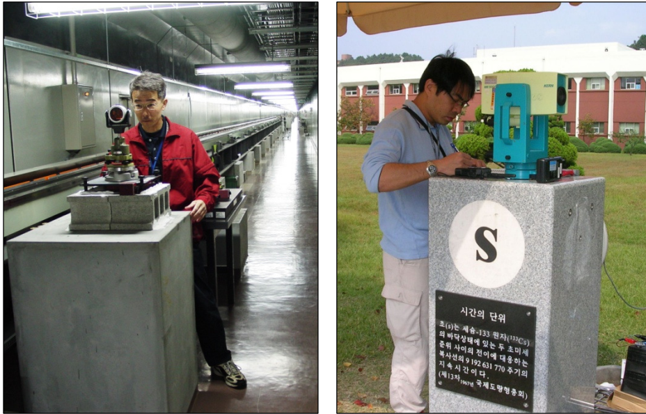
Figure 9.14 EDM comparisons in Asia. Left: tacheometer reflector on a pillar and rail constructions at the NMIJ laboratory tunnel in Tsukuba, Japan. Right: Mekometer measurements on pillar “s” at the KRISS geodetic baseline in Daejeon, Republic of Korea. The seven monuments have the names and contain definitions for the seven SI base units.
