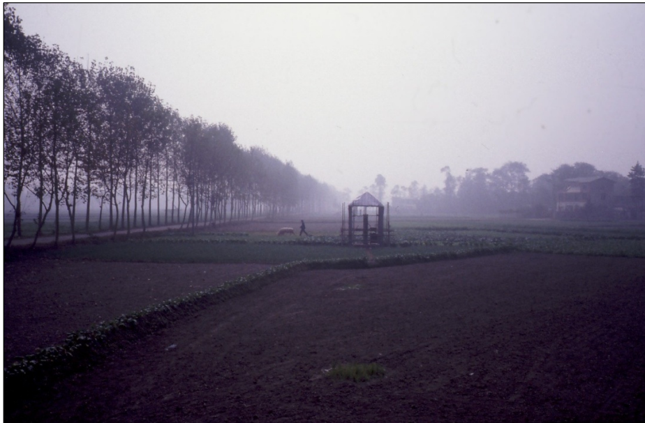
Figure 5.7 The southern part of the Chengdu Standard Baseline, with a new pillar at 96 m in front.
