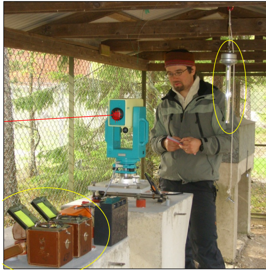
Figure 9.1 Measuring for calibration of the Kern Mekometer ME5000 at the 0 pillar of the Nummela Standard Baseline, with two Thommen aneroids, bottom left, and a suspended Assmann psychrometer, top right.
