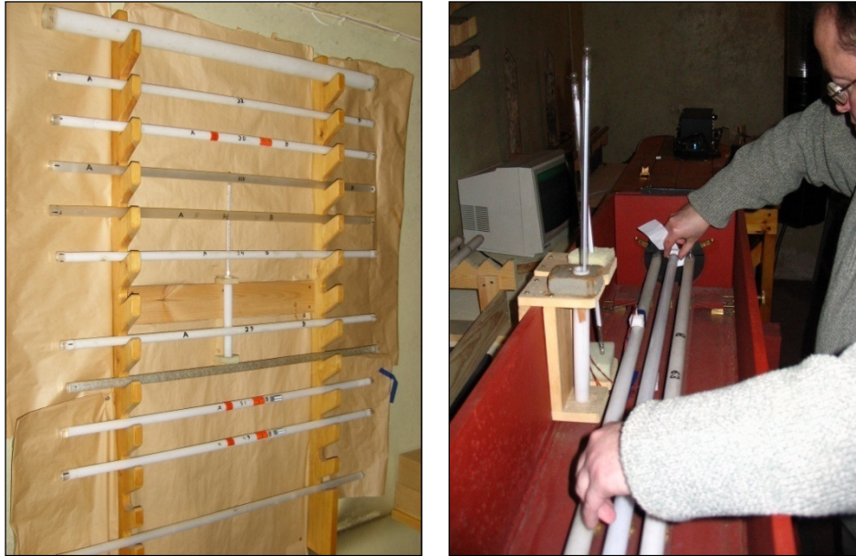
Figure 3.1 Some of the most frequently used quartz gauges at Tuorla (left), and tuning a middle quartz gauge in the comparator “Saunapiano”. The side quartz gauges no. 63 and no. 64 are used to control the parallelism of the end planes.
