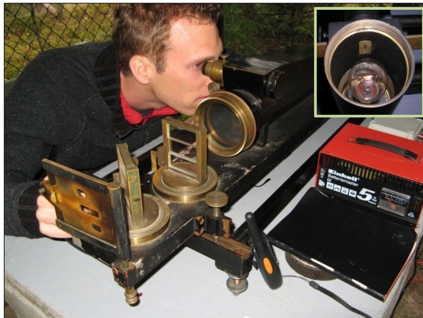
Figure 4.8 Searching for interference fringes by adjusting the screen and turning the compensator glasses in front of the telescope. A detail of the lamp at the top right.
