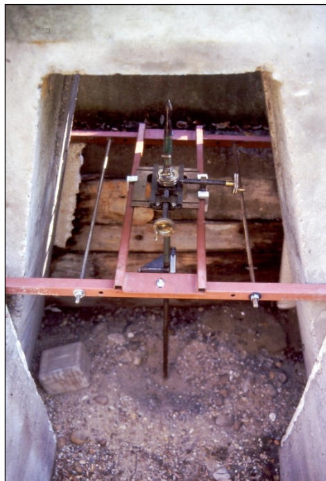
Figure 6.5 The plumbing rod equipment on an underground marker.
