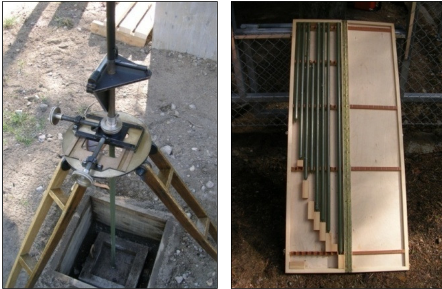
Figure 4.22 A plumbing rod with two levels is adjusted above an underground marker using a special tripod with a stage slide system (left). A set of adaptor bars can be used to adjust the height of the plumbing rod (right).
