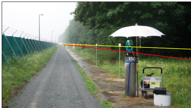
Figure 9.10 PTB's Geodetic Baseline with environmental sensors in Braunschweig, Germany. The fence on the left is for safety when measuring with lasers.
