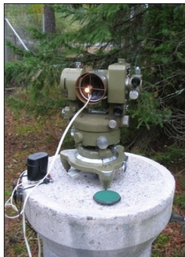
Figure 4.4 Kern DKM3 theodolite with an autocollimation lamp on the theodolite pillar.
