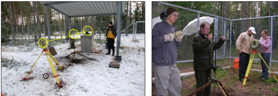
Figure 4.21 Arrangements for projection measurements. The theodolite and the (top of the) adjustable plumbing rod are set up at about the same height as the mirror centre and perpendicular to the baseline (left). Marking the location of the theodolite with a wooden stick in the ground helps with finding the best location for later measurements. Four persons are needed for a properly performed tape measurement: two people holding the tape at a constant strain and two people reading it (right).
