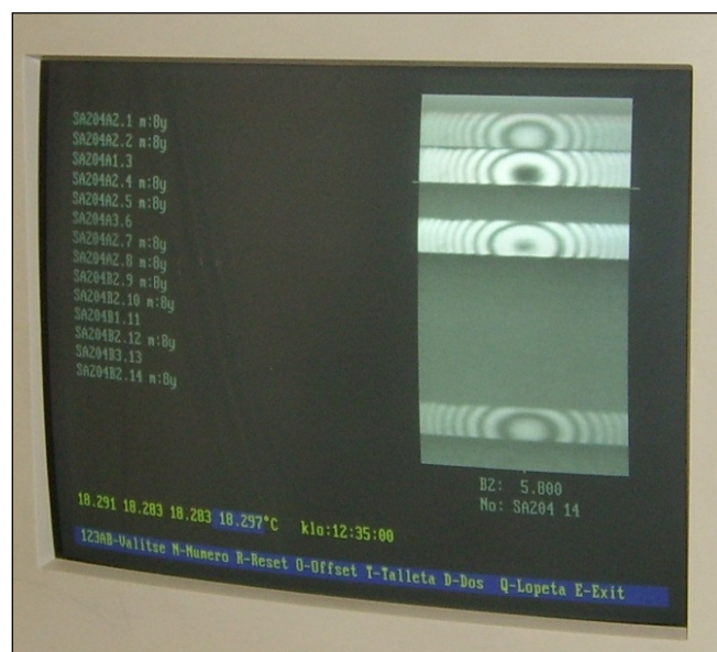
Figure 3.5 A picture of the B-end of quartz gauge no. VIII in the up position. The cameras, computers and monitors will be replaced with modern ones by 2014.
