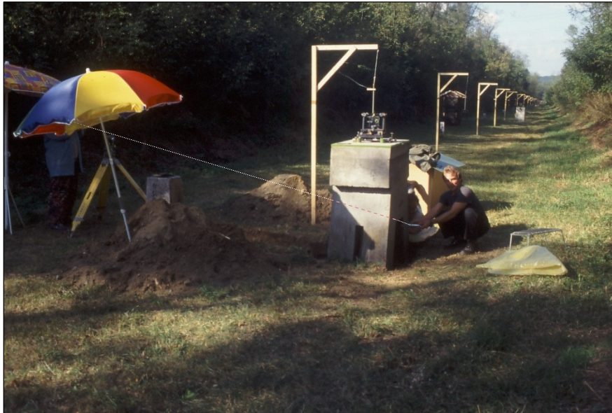
Figure 6.4 Tape measurements for projection at pillar 24.
