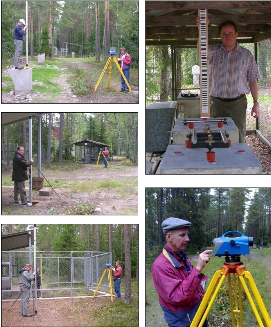
Figure 4.2 Arrangements for precise levellings with a Zeiss DiNi12 digital level and two bar code rods. The height differences between the underground markers are levelled first, both to and fro. The height differences between the underground markers and the reference points on the observation pillars are levelled next. Common levelling accessories and auxiliary pillars are used as intermediate points. Rulers or homemade bar code rods may be needed to determine the heights of the observation instruments.
