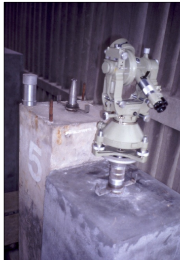
Figure 5.11 The central marker of pillar no. 5 and the Wild T3 fixed on the forced-centring plate on the new theodolite pillar. The theodolite was used in alignment of the mirrors.
