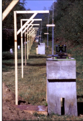
Figure 4.16 Line of thermometers along a standard baseline, next to the line of mirrors on observation pillars (photo from Gödöllő, Hungary, in 1999).
