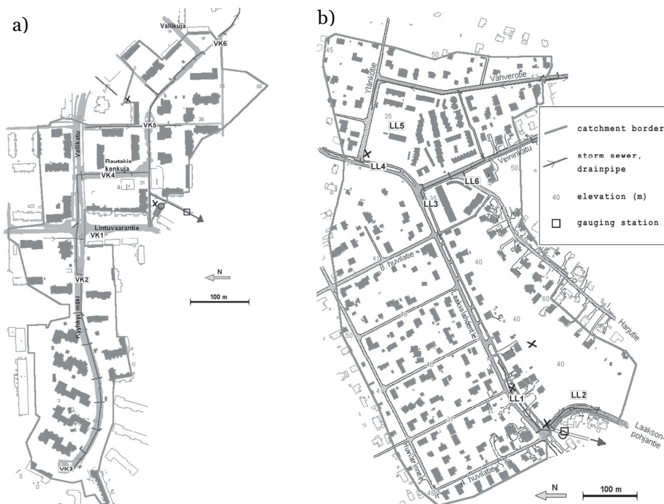
Figure 3. Illustrations of a) the medium-density VK catchment and b) the low-density LL catchment showing the locations of the main roads, buildings, pipe sewers, and the gauging stations (Sillanpää and Koivusalo, 2013, reprinted with permission from IWA Publishing). Also the locations of the snow courses used in the snow surveys are shown: the snow courses VK1-VK6 in VK and the snow courses LL1-LL6 in LL. The locations of open ditches in LL are not shown.
