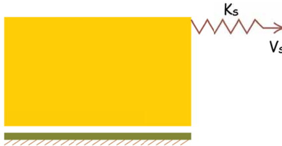
Figure 2.3. A block sliding on a flat substrate. A spring is attached to the block and the "free" end of the spring moves with the velocity v_s .
