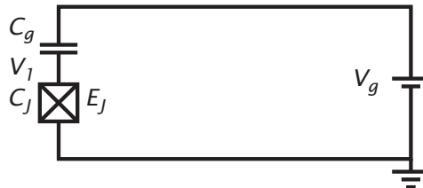
Fig. C.1: Circuit diagram of the simplified system.
