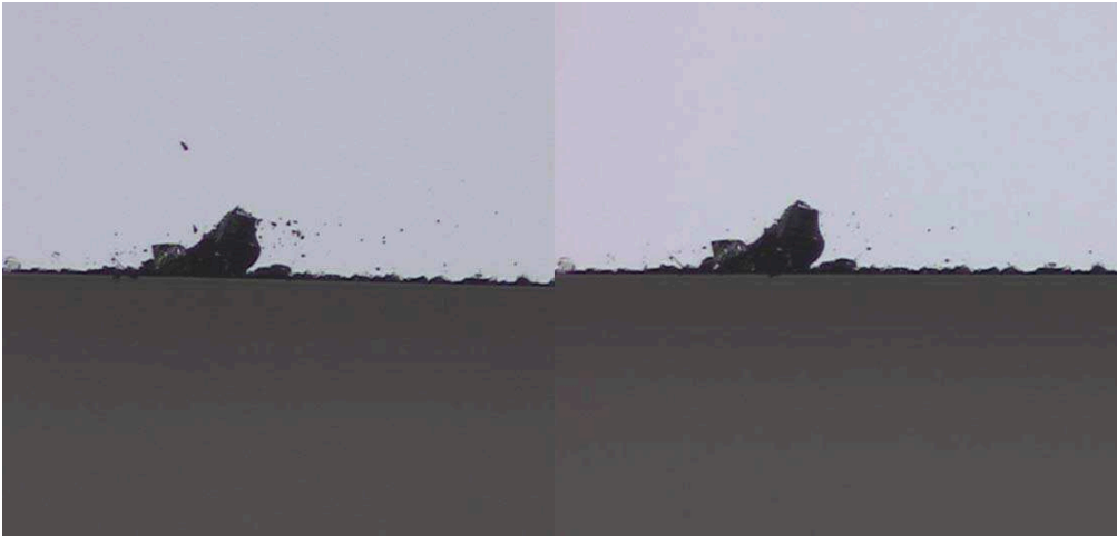
Fig. F.1: Cleaning a silicon chip in a spinner. On the left, a silicon chip edge prior to cleaning. On the right, a chip after spinning at 6000 rpm and rinsing with IPA. Most of the silicon particles have been removed.
