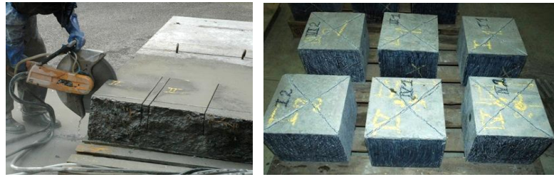
(a) The process of cutting the sample cuboids using a diamond saw. (b) The marking of cuboids by a milled cross and water resistant blue colour.
