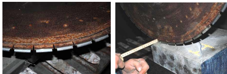
(a) The disc of a saw with diamond in-cisors. (b) The measuring of a slice.
