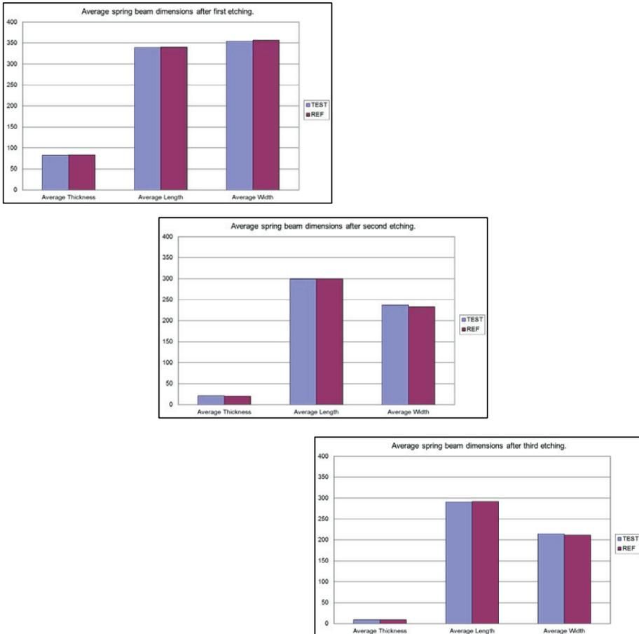
Fig 77. Etching results of Ultra Poligrind wafers (Test) compared with CMP polished wafers (Ref). Comparison of etching results shows that Ultra Poligrind wafers are equal (within the error limits) to CMP polished wafers.
