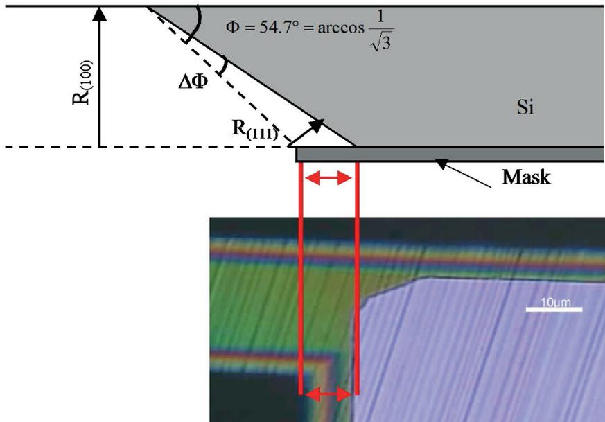
Fig 67. Schematic figure of direction  $\langle 111 \rangle$  under etching and optical microscope photograph of etched pillar with direction  $\langle 111 \rangle$   $\text{SiO}_2$  mask under etching.
