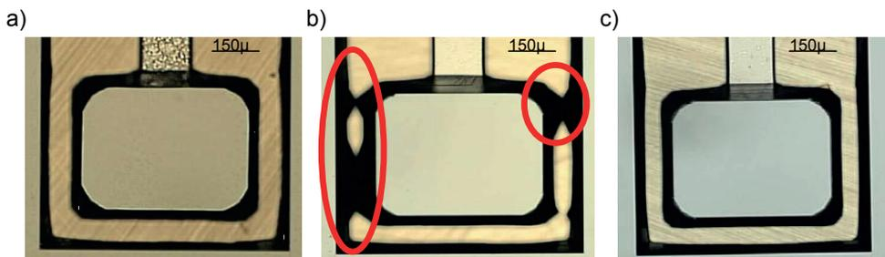
Fig. 63. Optical micrographs of etched seismic masses as a function of wafer oxygen level: (a) 15 ppma, (b) 10 ppma and (c) 7 ppma. Etching has failed in case (b) as evidenced by the discontinuous accelerometer frame.
