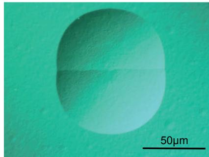
Fig 61. Microscope picture of anisotropic KOH wet etched single crystalline silicon wafer surface with wide twin etch pit induced by oxygen plasma.
