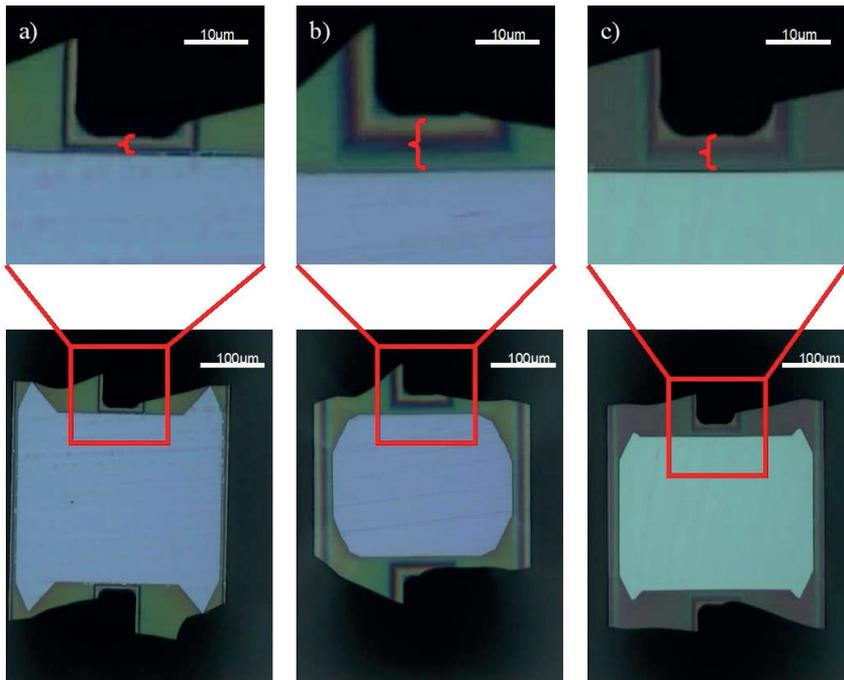
Fig 68. Optical micrographs of mask undercut: (a) fine grind wafer with 60 s KOH dip, (b) the fine ground wafer without KOH dip, (c) polished reference wafer.
