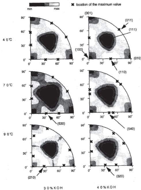
Fig 28. Fastest etching planes in a single-crystal silicon spherical in different temperatures and different concentrations [Sato 1997].
