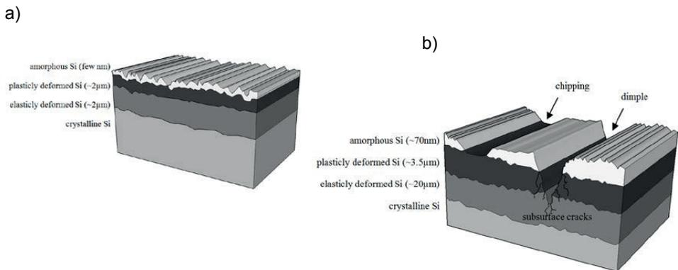
Fig 19. Damage models of FG-Si (a) and RG-Si (b) [redrawn from Yang Y 2008].
