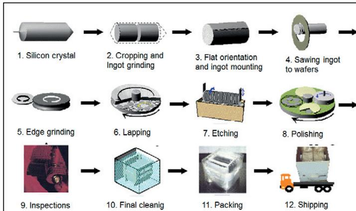
Fig 18. Flowchart of standard silicon wafering process.
