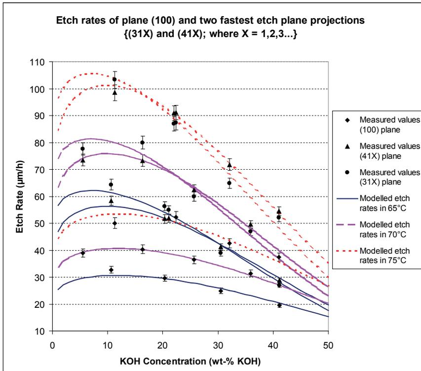
Fig 54. Etch rates of plane (100) and two fastest etch plane projections (31X) and (41X) (where X = 1,2,3...) as a function of KOH concentration. Compare Fig 10.
