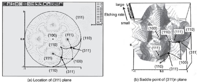
Fig 29. Distribution pattern of etching rate showing saddle point of (311) plane (34.0 wt-% KOH) [Shikida 2002].
