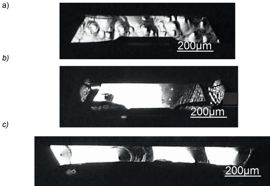
Fig 65. Optical micrographs of etched (111) planes (seismic mass walls) as a function of wafer oxygen level: (a) 15 ppma, (b) 7 ppma and (c) 10 ppma.
