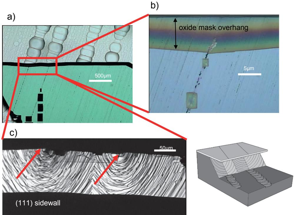
Fig 70. Ground wafer without KOH dip. Silicon etched 110 μm deep: (a) overview, (b) detail of mask undercut, (c) two large grooves result in rough (111) surface.
