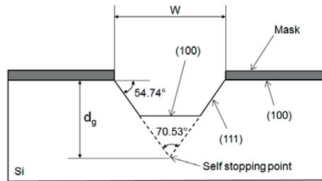
Fig 5. Anisotropically etched V-groove to (100) wafer, cross section.
