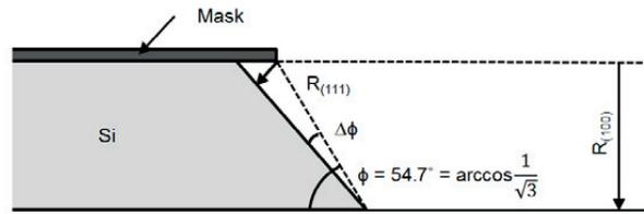
Fig 35. Etching of the (111) plane under mask oxide [redrawn from Lang 1996].
