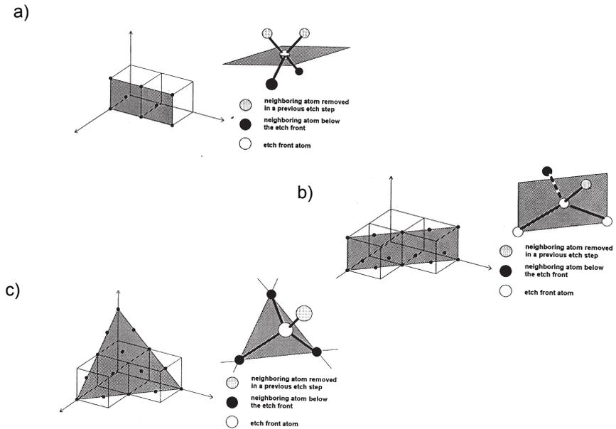
Fig 11. Positions of surface atoms, bound bonds and free bonds, in relation to the etch front. a. (100) b. (110) and c. (111) planes [Than 1994].
