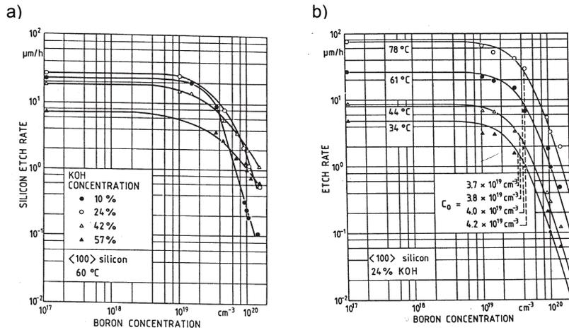
Fig 30. a. Change in the etching rate of the (100) plane as a function of boron doping concentration at different KOH concentrations [Seidel 1990 2]
