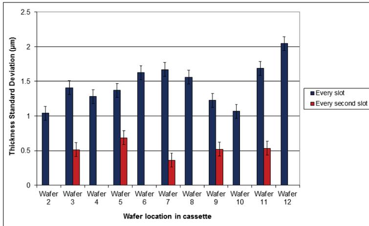
Fig 56. Influence of the distance between wafers in flow-through bath to etching results. Wide spacing led to beam thickness standard deviation across the wafer of 0.4–0.7 µm, while dense spacing resulted in 1–2 µm variation across the wafer.
