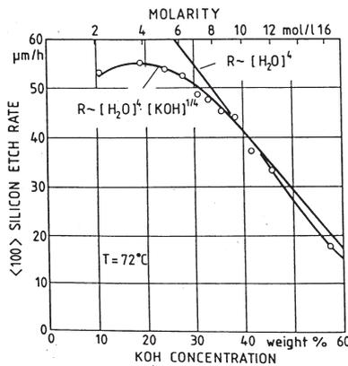
Fig 10. Etch rate of silicon (100) as function of the concentration of KOH etchant at 72 °C [Seidel 1990 1].
