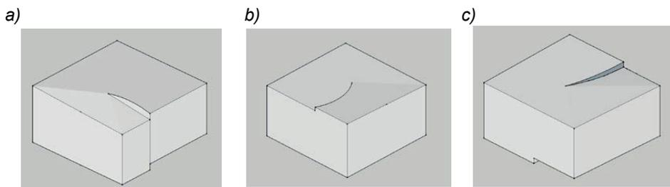
Fig 15. a. Step caused by screw dislocation. b. The step moves when a crystal is grown and c. The step moves when a crystal is etched [redrawn from Elwenspoek 1998].
