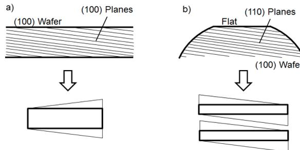
Fig 36. (a) Orientation error of the surface of the wafer makes a rectangular shape become tapered in anisotropic etching [adapted from Lang 1996]. (b) Orientation mistake of the flat surface causes a rectangular shape to become a parallelogram in anisotropic etching [redrawn from Lang 1996].
