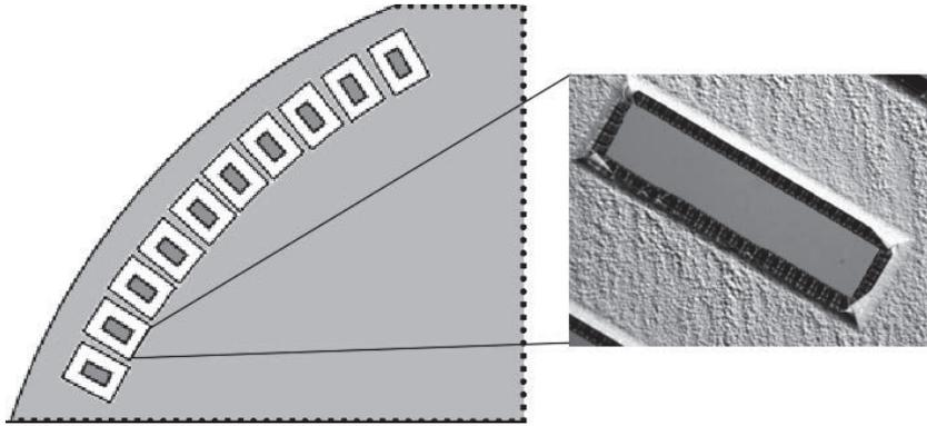
Fig 53. A test mask pattern of rectangular windows with subdivision into angles of  $3^\circ$  on outer circle of the wafer. An optical microscope picture of under-etched rectangular window in the enlarged picture.
