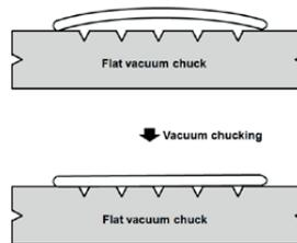
Fig 25. Removal of wafer bow by flat vacuum chucking [redrawn from Shimura 1989]
