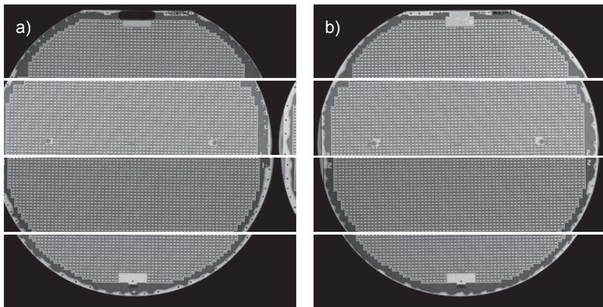
Fig 78. Scanning acoustic microscope images of the anodic bonded Ultra Poligrind grind structure wafer. (a) shows the number 1 side bonded surface and (b) shows the number 2 side bonded surface. Well bonded areas show as dark grey and non-bonded areas as white. As the figure shows, all cell frames are well bonded.
