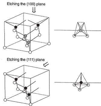
Fig 9. Difference of surface structure between plane (100) and plane (111) is shown. Etchant is in contact only with the atoms shown in black [Lang 1996].
