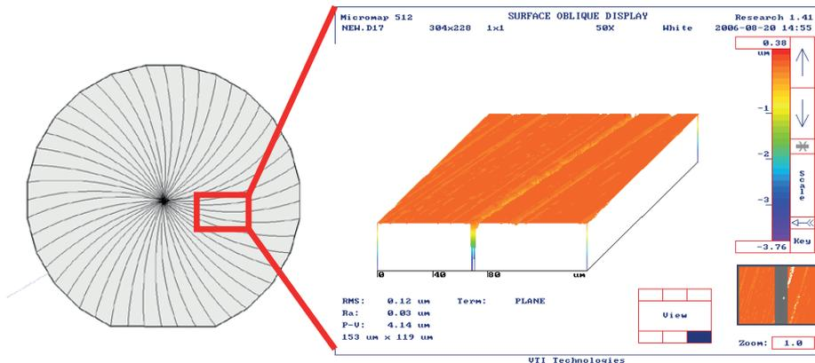
Fig 69. Optical profilometry map of a single deep groove after fine grinding and KOH dip. The depth is ca. 4  $\mu\text{m}$ .
