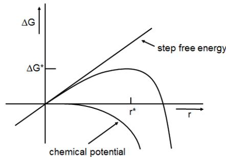
Fig 14. Free energy of the smooth surface as a function of the radius of the hole on the surface [redrawn from Elwenspoek 1998].
