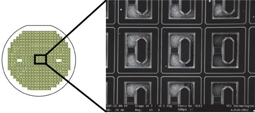
Fig 46. SEM picture of successfully etched anisotropic KOH wet etched single crystalline silicon seismic masses and spring beams in the wafer.
