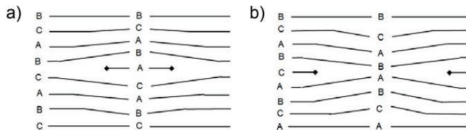
Fig 21. Stacking faults generated by excess atomic plane (a) or absent atomic plane (b). These are called Frank partial dislocations.
