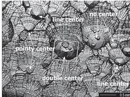
Fig 38. Typical overviews of the (111) plane wafer with etch pits after KOH etching. [Nijdam 2000].
