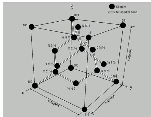
Fig 2. The unit cubical structure of the diamond lattice of silicon.
