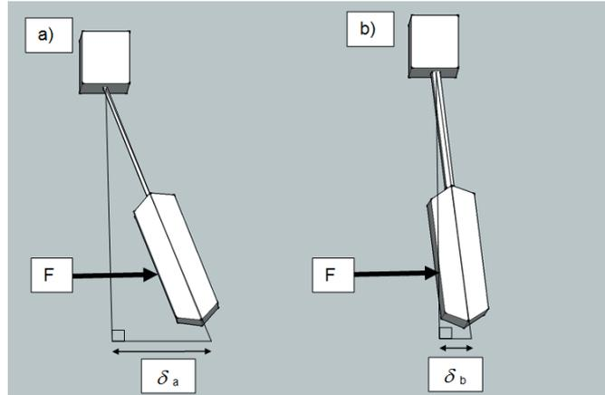
Fig 49. Schematic illustrations of two different elements with different beam dimensions show the same g-value. The mass with thinner, narrower or longer beam (a) will move more than the mass with thicker, wider or shorter beam (b) and cause more nonlinearity to the component.
