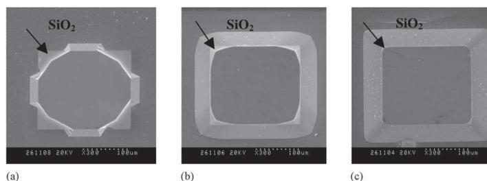
Fig 31. Convex figures etched in (a) 10M KOH solution ( $t = 30$  min), (b) 5M KOH + IPA solution ( $t = 60$  min), and (c) 5M KOH + tert-butanol solution ( $t = 60$ min) [Zubel 2002].
