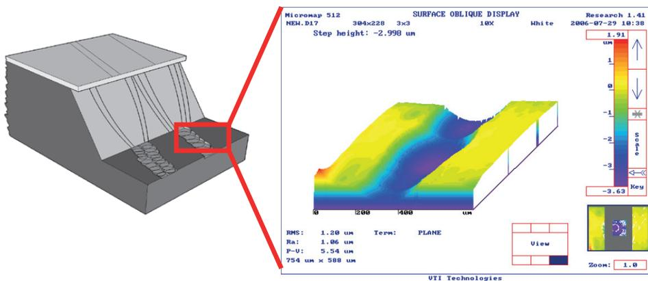
Fig 72. Optical profilometry map of a groove in the etched bottom (110 μm from the surface). Depth of the groove is about 3 μm. This is comparable to 4 μm depth measured for ground wafer. The width of the spherical depressions is from 200 μm to 300 μm. This is much wider than for the untreated case, and results from the deep KOH etching.
