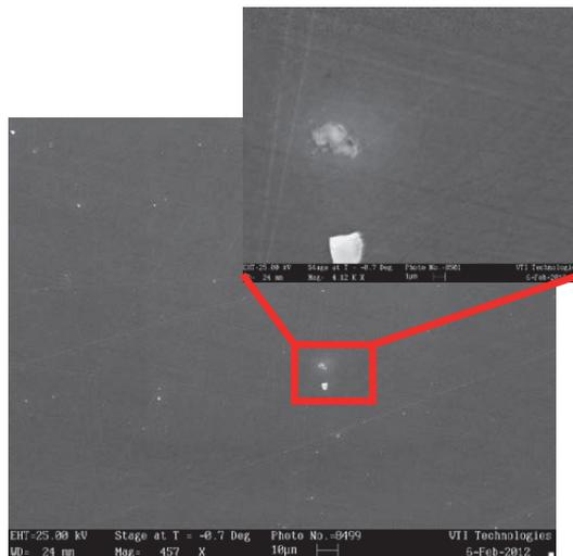
Fig 73. SEM picture of Ultra Poligrind wafer surface which shows shallow grinding lines and other shallow scratches.
