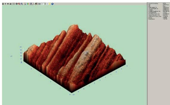
Fig 75. After about 1.2  $\mu\text{m}$  oxidation process the Ultra Poligrind surface roughness is decreased below 1 nm in 10 x 10  $\mu\text{m}$  measurement area in AFM analysis software tool, Nova map.
