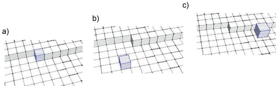
Fig 12. Behaviour of the atom in an active position in the etching ( $a \rightarrow b \rightarrow c$ ) and in the growth of the crystal ( $c \rightarrow b \rightarrow a$ ) [redrawn from Elwenspoek 1998].
