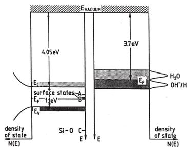
Fig 8. Silicon and KOH electrolyte energy band structure and electron affinity before contact [Seidel 1990 1].
