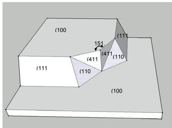
Fig 27. The convex corner under-etching and formation of the fastest etching plane [redrawn from Mayer 1990].
