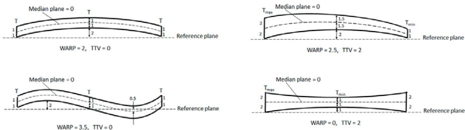
Fig 26. Deformed wafer shapes with related Warp and TTV [redrawn from Shimura 1989]
