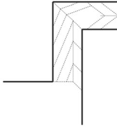
Fig 42.  $\langle 110 \rangle$  direction corner compensation figure, which has the form of L and its etching behaviour.
