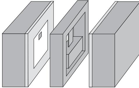
Fig 45. Schematic figure of a bulk micromachined accelerometer: anisotropic KOH wet etching defines the single crystalline silicon seismic mass and spring beam in the middle wafer
