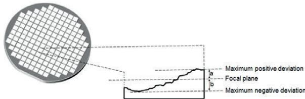
Fig 23. Local site flatness for wafer divided into exposure arrays [redrawn from Shimura 1989].
