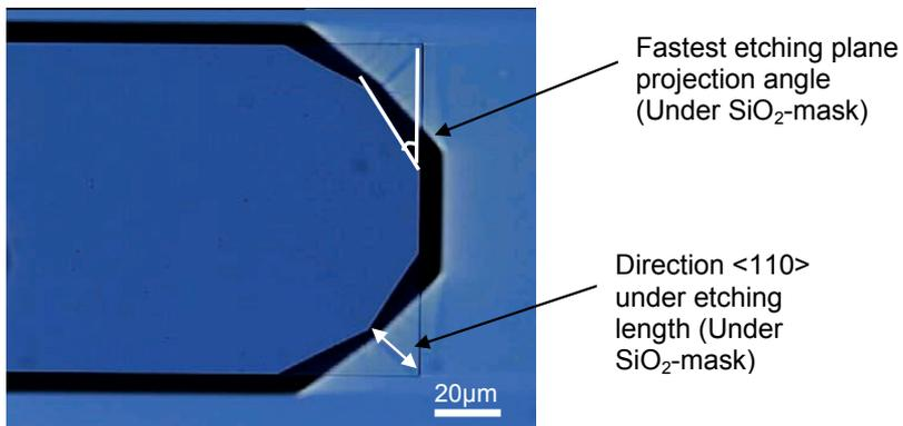
Fig 51. Anisotropically etched figure and the measured dimensions: projection angle of fastest etching plane and direction  $\langle 110 \rangle$  under etching length.
