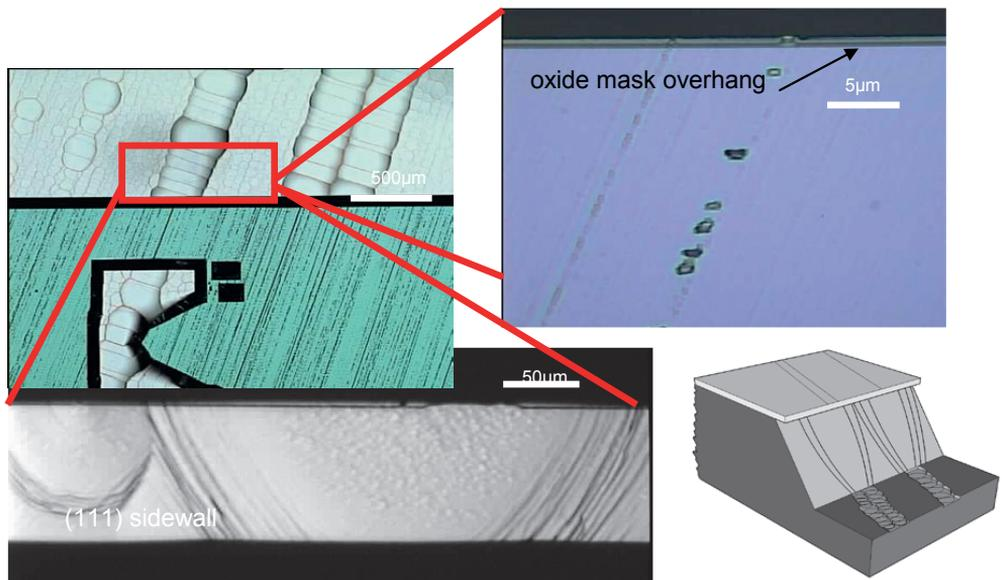
Fig 71. Greatly reduced undercutting and improved (111) surface smoothness in KOH-dipped ground wafer.
