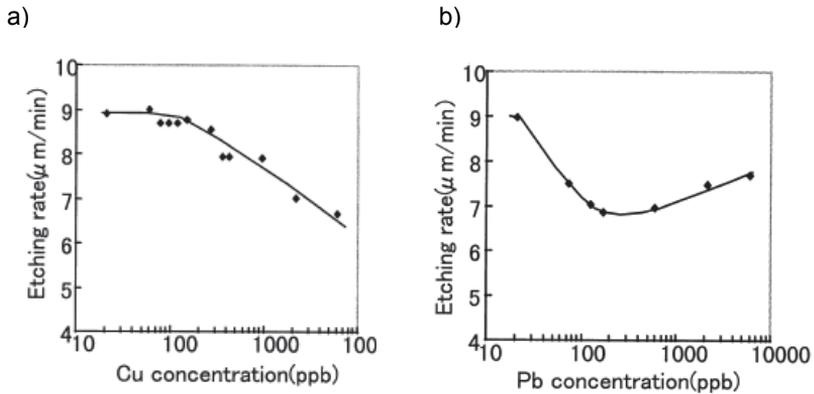
Fig 34. Etching rate of p-type Si (110) versus (a) concentration of Cu and versus (b) concentration of Pb (110 °C and 32 wt-% KOH) [Tanaka 2000].
