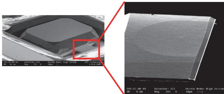
Fig 60. SEM picture of anisotropic KOH wet etched single crystalline silicon seismic mass and spring beam. In the spring beam, there is a shallow etch pit caused by ( $\text{Fe}_x\text{O}_y$ ) particles.
