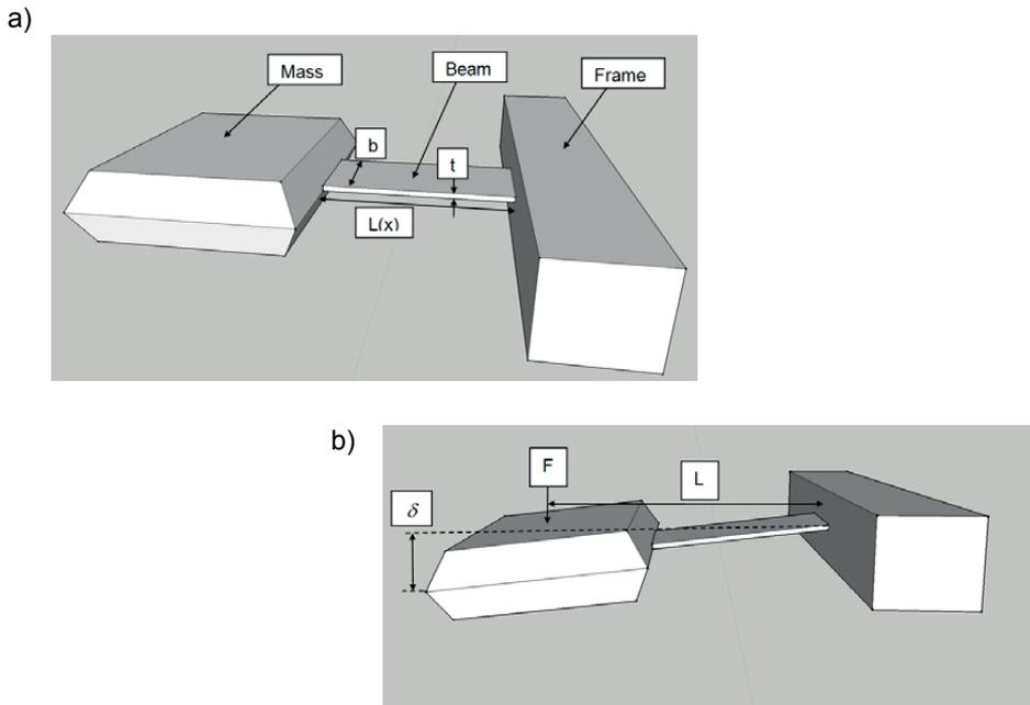
Fig 47. (a) Schematic representations of the accelerometer seismic mass and spring beam dimensions
