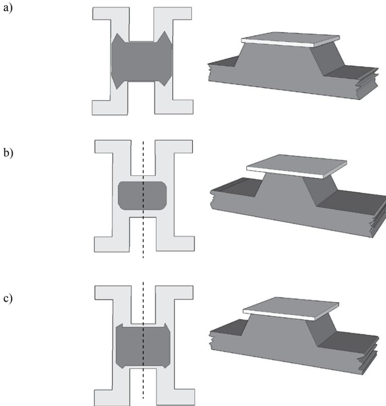
Fig 44. Author corner compensation design and the resulting mask undercut from chapter 7.2: (a) a fine ground wafer with 60s KOH etching, (b) a fine ground wafer without KOH etching and (c) reference polished wafer. The 3D drawing shows a cut along the dotted line.
