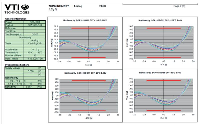
Fig 48. Centrifuge nonlinearity measurement results of analog 2g SCA1020 sensor component. Measurements show the seismic mass move (Vout change) from -3g to +3g. To pass result the Vout (mg) should be in the specification (+/-45mg) in the whole measurement area (-1.7g to +1.7g) and at all temperatures.
