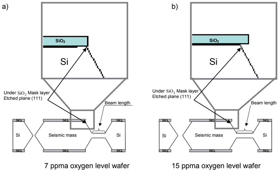
Fig 62. Schematic of seismic mass (111) sidewall plane etching under SiO<sub>2</sub> mask for two oxygen levels: under-etching is more serious in the case of oxygen level of 15 ppma (a) than for 7 ppma (b).
