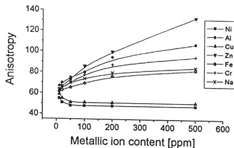
Fig 32. Anisotropy of silicon as function of the amount of metal impurities in KOH solution [Hein 1997].
