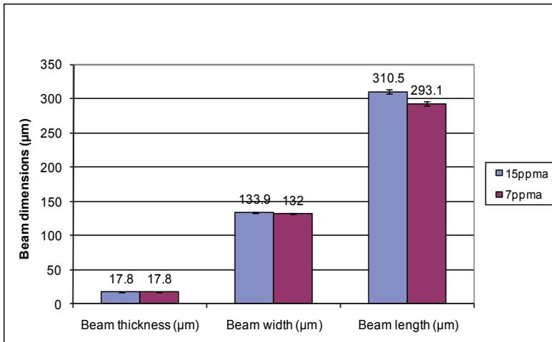
Fig 64. Beam thickness, beam width and beam length of MCZ wafers with high oxygen level (15 ppma) and low oxygen level (7 ppma). The results for 10 ppma beams are not shown because of failed etching.
