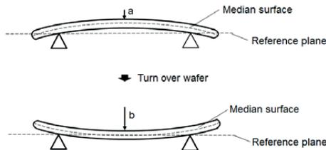
Fig 24. Wafer bow and its measurements [redrawn from Shimura 1989].
