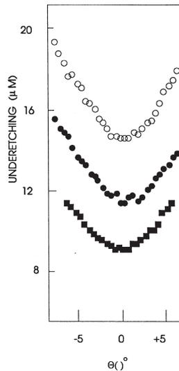
Fig 16. Under-etching of (111) plane as a function of the corner mistake in KOH etchant (40%). White circles: 30 °C, 300 min; black rectangles 70 °C, 15 min; black circles 108 °C, 3 min [Elwenspoek 1994].
