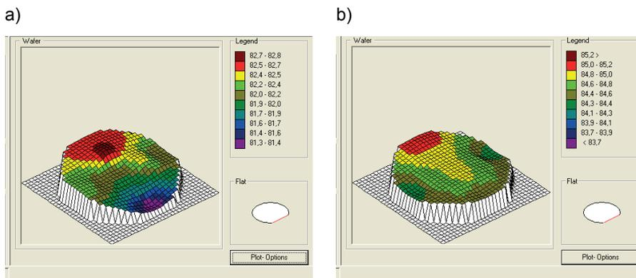
Fig 59 (a) Beam thicknesses near the flat of the wafer are thinner than on the wafer top ( $\sigma = 0.57\%$ ) in the flow-through bath. (b) In the rotational flow bath the beam thickness uniformity is much improved ( $\sigma = 0.37\%$ ).
