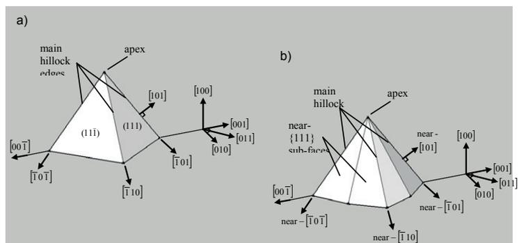
Fig 37. Schematic figures of hillocks. (a) a hillock having (111) plane side walls and (b) a hillock whose side walls are close to the (111) plane, for example, {567} plane [redrawn from Landsberger 1996].
