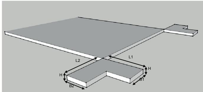
Fig 43. 3D schematic view of the corner compensation layout, which yields the most desired free end corners [redrawn from Biswas 2006].
