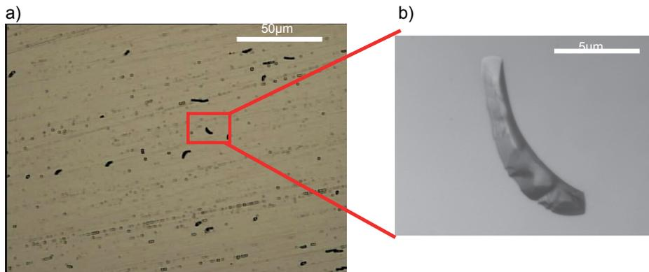
Fig 20. Fine-grind silicon surface, preferential etched with KOH (20 wt-% and 60 °C) for 60 s, which still has subsurface damage caused by coarse grinding.
