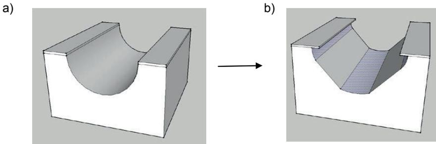
Fig 41. (a) Cylinder-shaped hole. (b) The faster etching planes (the violet areas) and the planes that etch more slowly form the walls of the hole [adapted from Elwenspoek 1994]
