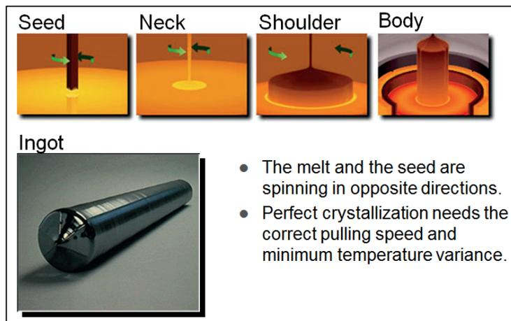
Fig 17. Single-crystalline silicon pulling by the Czochralski (CZ) Method.
