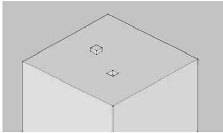
Fig 13. To loosen one atom in the (111) plane, three strong bonds must be cut from the plane ( $3\phi$ ). The energy of one bond is obtained from the back binding ( $\phi$ ) [redrawn from Elwenspoek 1998].
