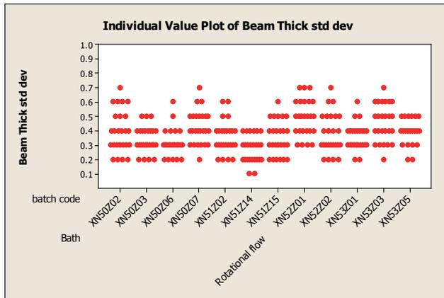
Fig 58. Variation in standard deviation of beam thickness over 10 batches in two baths each (25 wafers in one batch): (a) flow-through bath  $\sigma = 0.4\text{--}0.7 \mu\text{m}$ ; (b) rotational flow bath  $\sigma = 0.3\text{--}0.4 \mu\text{m}$ .
