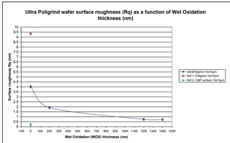
Fig 76. AFM measurement of surface roughness (Rq) of Ultra Poligrind ground wafers as a function of wet oxidation thickness. During the 1200 nm wet oxidation step the surface roughness decreases from 4 nm (Rq) to below 1 nm (0.74 nm Rq). The figure also shows the results of AFM measurement of surface roughness (Rq) of two reference wafers.
