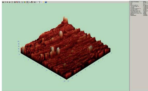
Fig 74. The Ultra Poligrind surface roughness is about 4 nm Rq-roughness (about 3 nm Sa-roughness) in 10 x 10  $\mu\text{m}$  measurement area in the AFM analysis software tool, Nova map.
