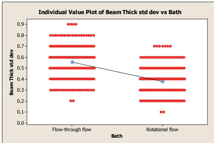
Fig 57. Comparison of accelerometer beam thickness between flow-through and rotational designs. The standard deviation of beam thickness for the rotational bath is  $0.38 \mu\text{m} \pm 0.13 \mu\text{m}$  (292 wafers; 2628 data points) and for the flow-through bath  $0.51 \mu\text{m} \pm 0.16 \mu\text{m}$  (165 wafers, 1485 data points).
