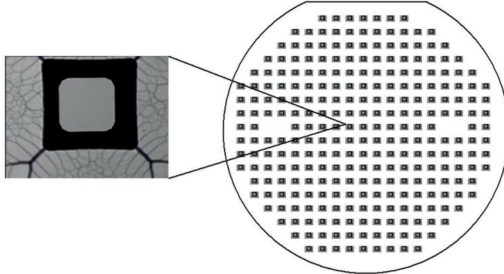
Fig 66. KOH etched silicon pillars in accelometer capping wafer.
