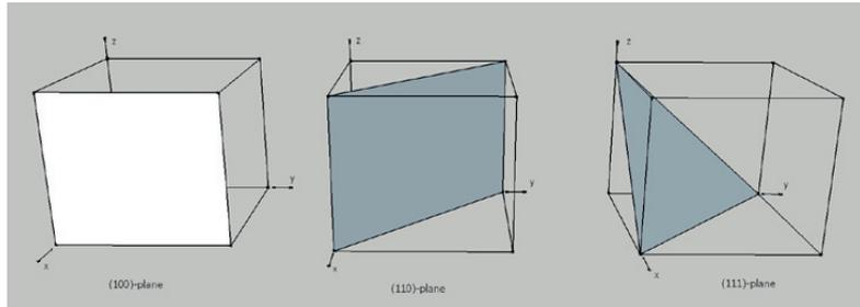
Fig 3. The most important crystallographic planes of the silicon.
