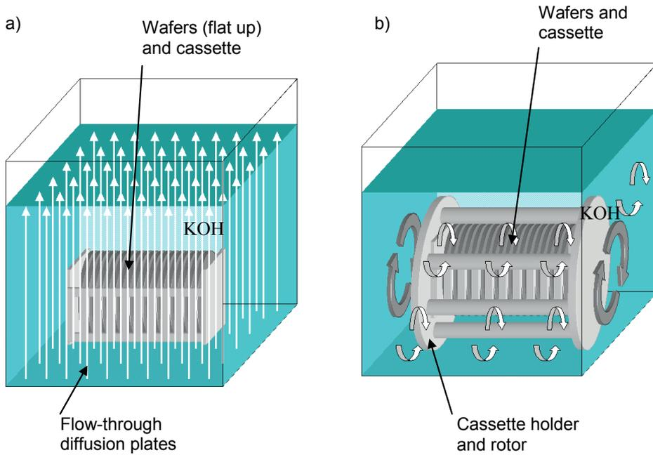
Fig 55. Schematic figures of (a) flow-through wet etching bath and (b) rotational flow wet etching bath.
