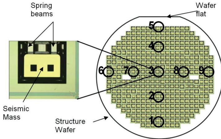
Fig 50. Anisotropically etched seismic masses and two spring beams of an accelerometer and laser profilometer measurement sites (numbered black circles) across the wafer.
