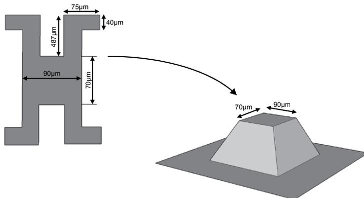
Fig 52. Corner compensated silicon test structure after ideal etching.
