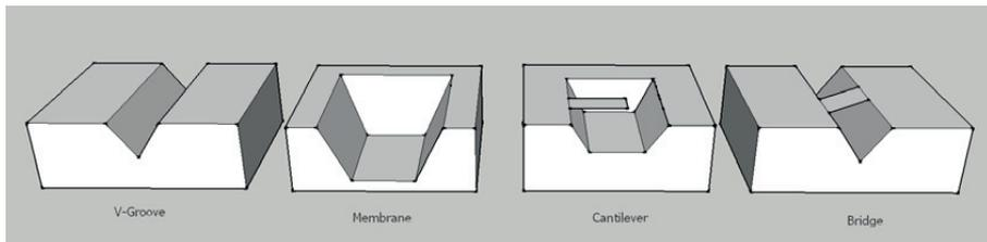
Fig 4. Structures accomplished by anisotropic etching to silicon wafer.
