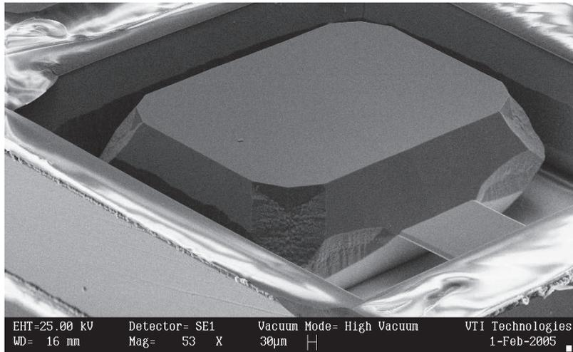
Fig 1. SEM figure of anisotropic KOH wet etched single crystalline silicon seismic mass and spring beam (cantilever) of bulk MEMS accelerometer sensor.
