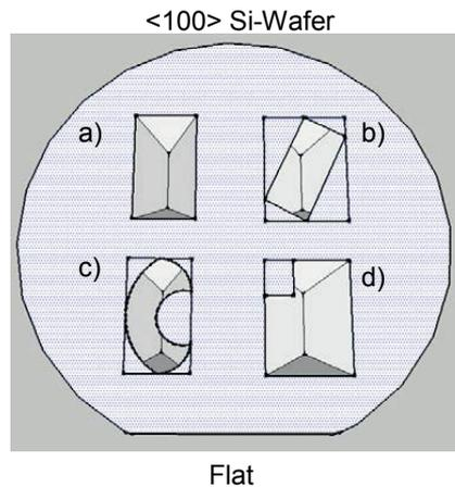
Fig 6. Figures anisotropically etched on the surface of the (100) wafer. Dotted area: figures made on the mask. Black line: figures accomplished with etching.
