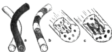
Scheme 8. The possible morphologies of bicomponent fibres according to Bognitzk. a) fibres consisting of the pure polymers, fibres composed of sequences of individual polymers, c) matrix-dispersed or co-continuous phase morphologies with dimensions smaller than the fibre diameter. 198
