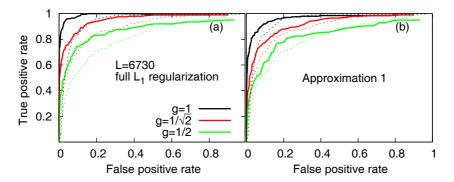
Fig. 4.4: ROC curves for full  $L_1$  regularization (left, solid lines) and Approximations 1 (right, solid lines) with  $g=0.5,\,1/\sqrt{2},\,1$  respectively. The green lines for g=0.5, red for  $g=1/\sqrt{2}$  and black for g=1. Corresponding dashed lines are for J0-cut method of these gs. The length of the data is L=6730.
