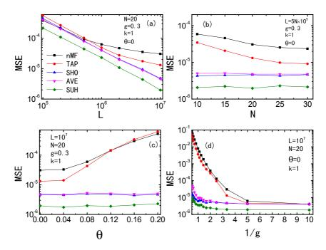
Fig. 3.1: Mean square error (MSE) versus (a) data length L, (b) system size N, (c) external field  $\theta$  and (d) temperature 1/g. Black squares show nMF, red circles, TAP, blue up triangle SHO, pink down triangle AVE and green diamond SUH, respectively. The parameters are g=0.3, N=20,  $\theta=0$ , L= $10^7$  except when varied in a panel.
