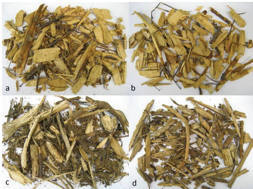
**Figure 6.** Raw materials before and after the screening: a) unscreened and b) screened HW biomass; c) unscreened and d) screened SW biomass. Accepted particles were collected from screens Ø7 and Ø13 mm.
