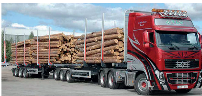
Figure 2.11. A 76t heavy vehicle combination: tractor + swap body + link + semitrailer.
