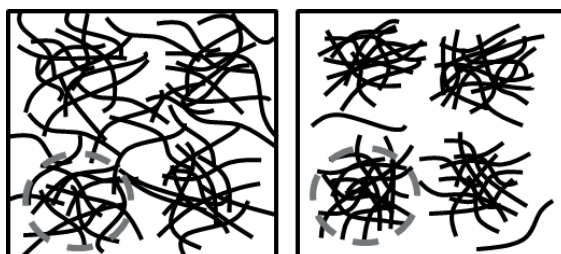
Figure 3. Schematic representation of the flocs in the fiber network at rest (on the left) and as individual entities under flow (on the right).
