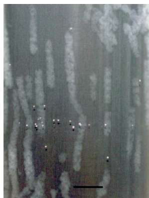
Figure 13. 0.1% MFC suspension immediately after shearing the suspension at apparent shear rate 0.5\text{ s}^{-1} for 10 min (paper I). The length of the scale bar is 5 mm.
