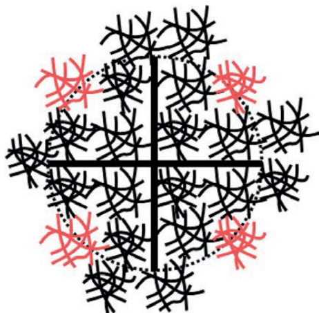
Figure 6. Schematic presentation of four-bladed vane rotor in a flocculated suspension. As the suspension yields, flocs inside the dashed line start to flow and the others stay stationary. Red flocs must either rupture or move and deform, while breaking contacts with neighboring flocs. Adapted from Mosse et al. 71 .
