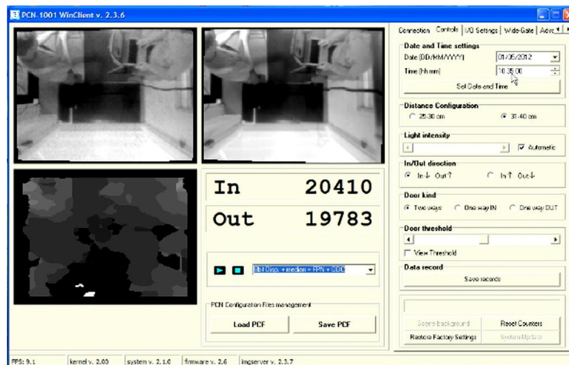
Figure 57. Configuration software of the Eurotech stereoscopic camera sensor. The two upper left views display the images acquired from the two cameras of the sensor and the view below shows the current tracking process and the disparity map.
