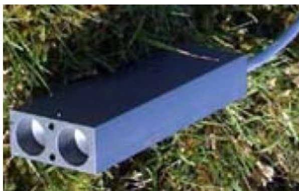
Figure 5. EcoCounter dual PIR sensor (Greene-Roesel et al. 2008).
