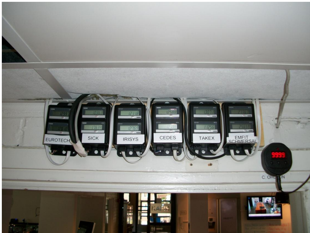
Figure 54. Indicators for cumulative counting monitoring. For direction sensitive sensors, the upper reading represents the “to café” and the lower the “to corridor” direction.
