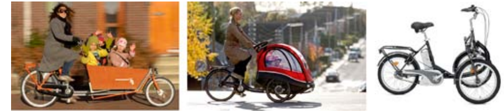
Figure 10. Special bikes could replace personal passenger cars in city traffic. Two- and three-wheeled cargo bikes offer transport capacity, and three-wheeled electrically-assisted bikes could offer independent travel for the elderly [33].
