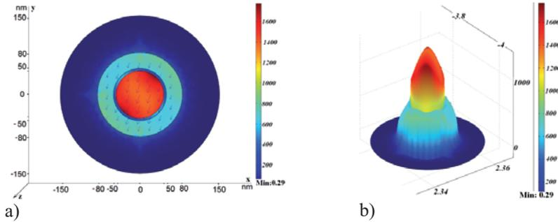
Fig. 29. Cross-section of the annular waveguide (a) and power flow distribution (b).
