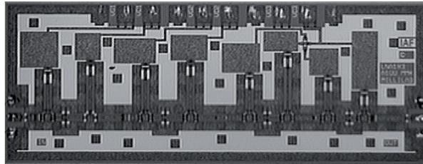
Fig. 18. Chip micrograph of the 183-GHz metamorphic HEMT low noise amplifier. The circuit area is  $2.5 \text{ mm}^2$  ( $2.5 \text{ mm} \times 1.0 \text{ mm}$ ).
