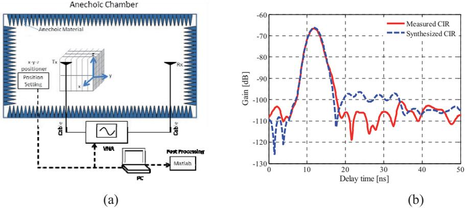
Fig. 4. (a) Measurement set-up in an anechoic chamber (b) Synthesized CIR vs. measured CIR, by using a bicone antenna at both Rx and Tx sides.
