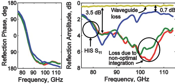
Fig. 20. Measured  $S_{11}$ -parameter of the reflection type phase shifter with MEMS tunable HIS over W-band. Reflection phase is  $0^\circ$  at the resonance frequency of 83.4 GHz. Minimum insertion loss of the HIS outside of the resonance is 0.7 dB.
