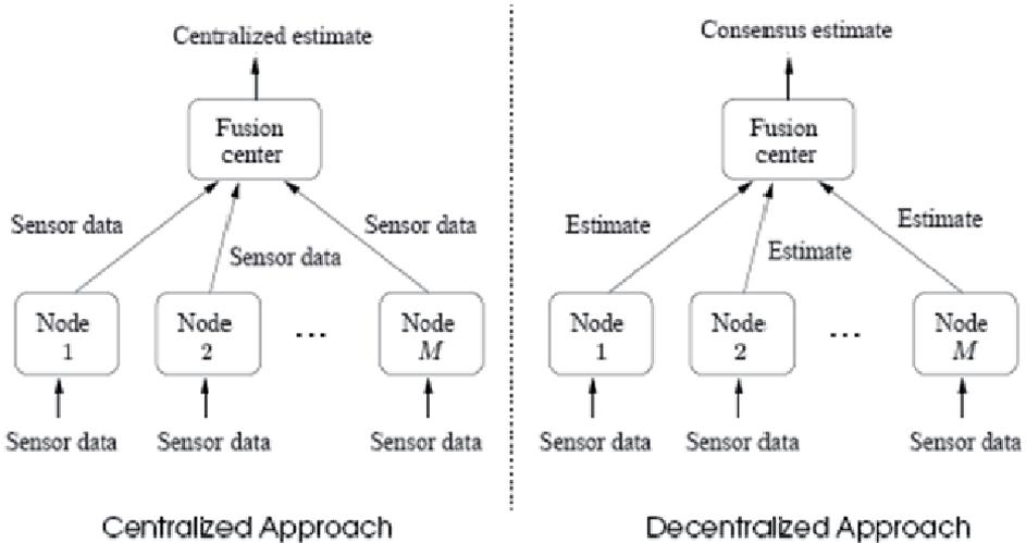
Fig. 6. Centralized and decentralized estimation in a network with  $M$  nodes.
