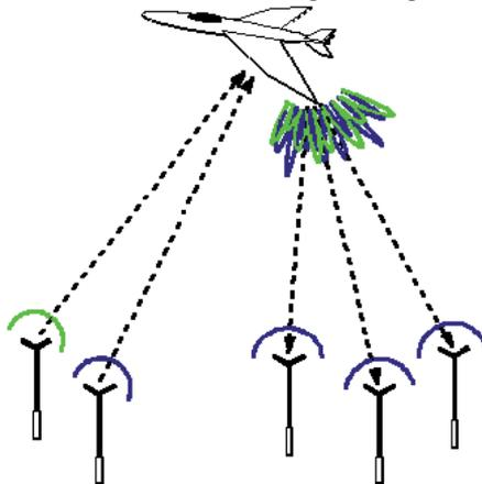
*Fig. 8. Multistatic, MIMO Radar configuration using waveform diversity. Virtual aperture may be created using signal processing for designing and optimizing the waveforms launched from each antenna.*
