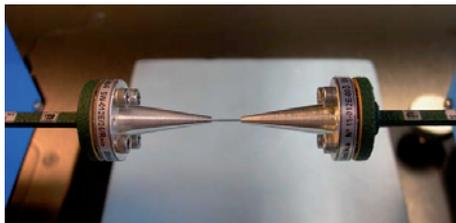
*Fig. 23. Measurement setup of a silicon rod waveguide at 220–325 GHz.*
