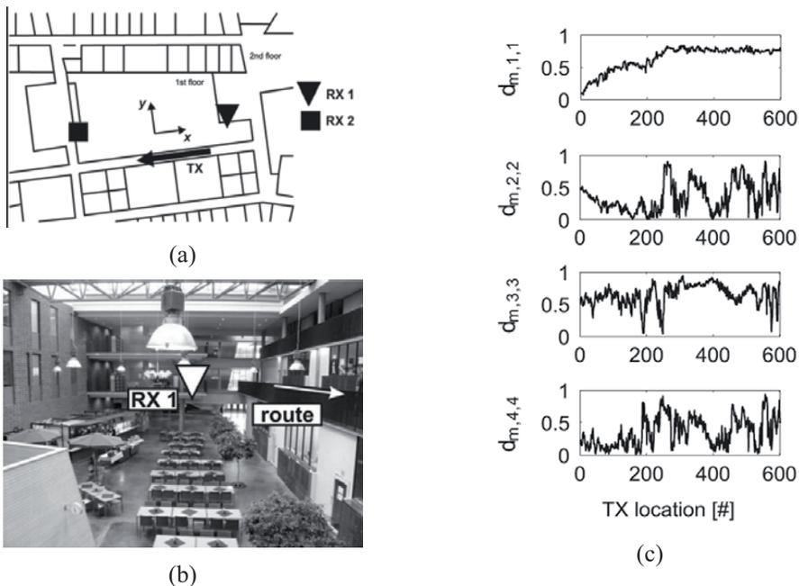
Fig. 3. (a) Floor plan and the coordinate system of the measurement, (b) photograph of the environment, and (c) correlation of the  $i$ th eigenvectors from the Tx-Rx1 and Tx-Rx2 links.
