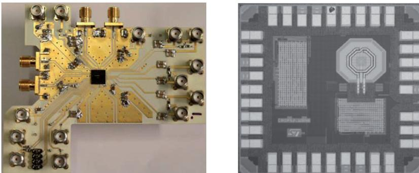
Fig. 14. a) Implemented wideband receiver b) Chip photograph of implemented synthesizer.
