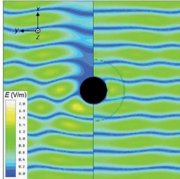
Fig. 9. Snapshot of simulated electric field when a plane wave hits an uncloaked (left) and a cloaked (right) object. The cloak is made of periodically stacked conical metal sheets.
