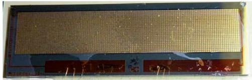
Fig. 21. Fabricated MEMS tuneable high-impedance surface for an analogue type phase shifter.
