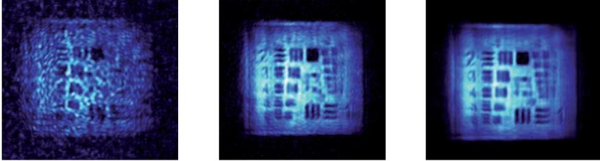
Fig. 26. Millimetre-wave image of USAF 1951 with system SNR of 0 dB, 10 dB, and 20 dB.
