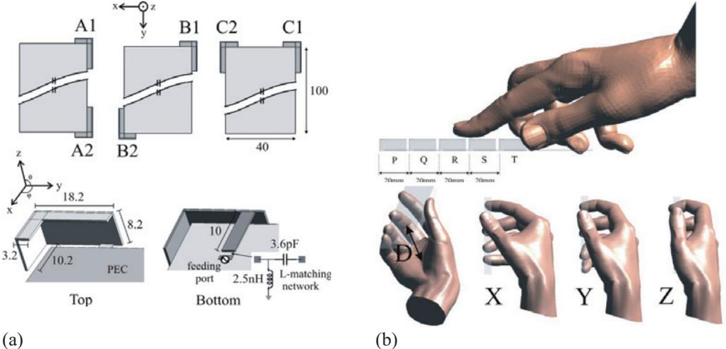
Fig. 16. (a) Coupling element –based dual-antenna structures with different configurations, (b) Multivariable study on hand effects.
