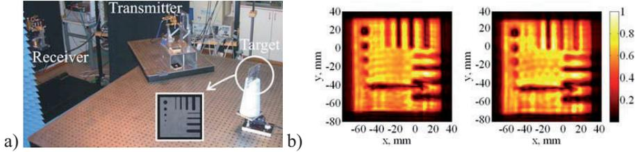
Fig. 25. Indirect holographic imaging. a) The setup. b) The images taken with holographic method (lhs) and with direct phase measurement (rhs).
