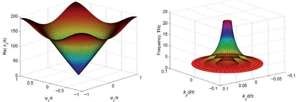
Fig. 30. Slow-wave factor for waves, propagating along CNTs over the transversal wave vector plane (isofrequency surface). b) Surface of dispersion for waves, propagating in a finite-thickness CNT slab.
