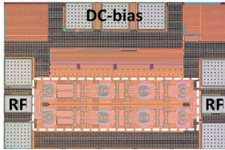
Fig. 17. Chip micrograph of the 94-GHz CMOS power amplifier. The area, including pads is  $0.24 \text{ mm}^2$  ( $610 \mu\text{m} \times 400 \mu\text{m}$ ) and the active area (encircled with the dashed white line) is  $0.069 \text{ mm}^2$  only.
