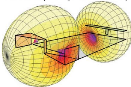
Fig. 1. Novel antenna structure with a capacitive coupling element (CCE, right) and a bow-tie antenna (left). The unbalanced (CCE) and balanced (bow-tie) antenna elements have almost orthogonal radiation patterns.
