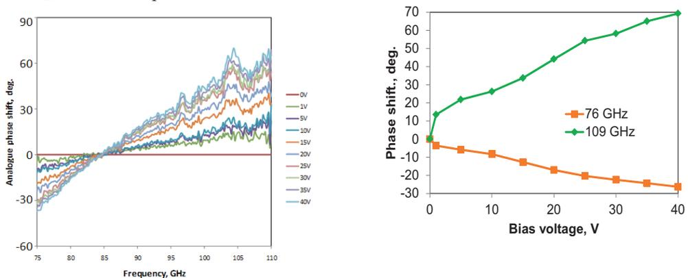
Fig. 22. Analogue type phase shift: frequency dependence for different bias voltages (lhs) and voltage dependence (rhs).
