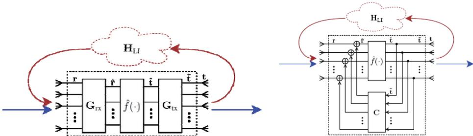
Fig. 5. Loop interference cancellation in spatial domain or subtraction of estimated loop interference.
