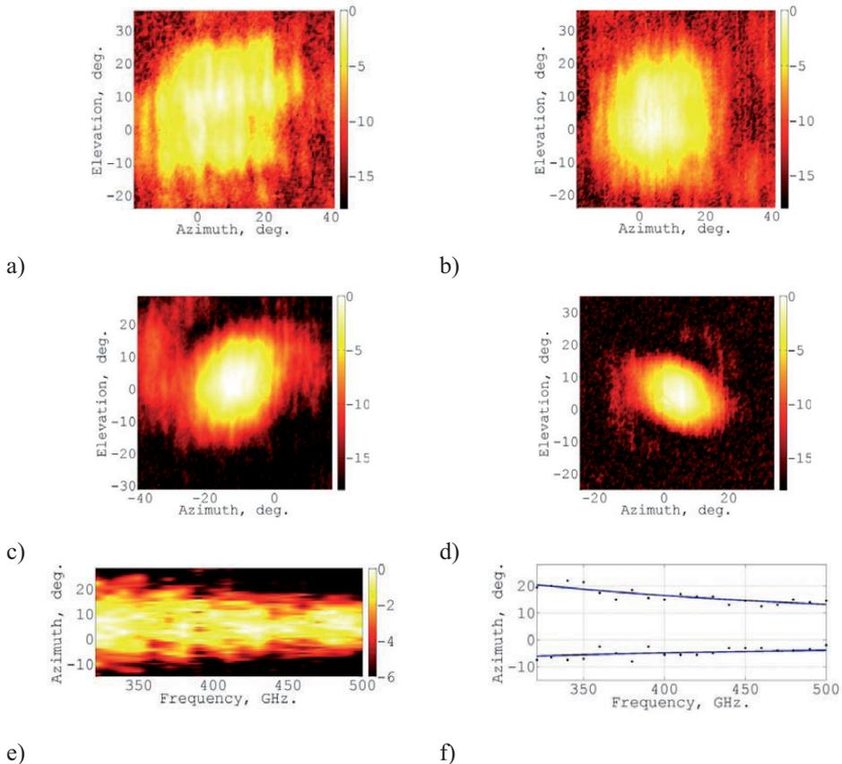
Fig. 28. Bolometer radiation pattern measurements at 321-850 GHz. (a-d) Radiation patterns at 321 GHz, 400 GHz, 654 GHz, and 780 GHz, respectively. (e) Azimuth cut of the radiation pattern at 321-500 GHz. (f) least squares fit to the radiation pattern cuts gives relation  $FWHM = 8.5^\circ$  per THz. The scales in the patterns are in decibels
