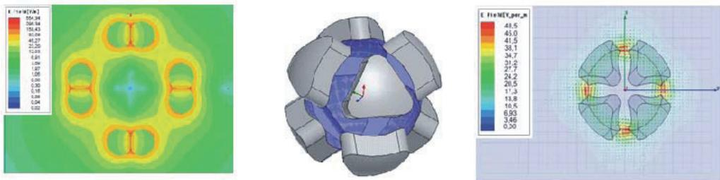
Fig. 34. (left) - Spatial distribution of the amplitude of electric field at 369 THz for an effective plasmonic loop comprising four dimers; (center) - A cluster made of eight triangular nanoprisms on a dielectric core; (right) - Spatial distribution of the electric field vector at 400 THz for the cluster comprising eight triangular nanoprisms.
