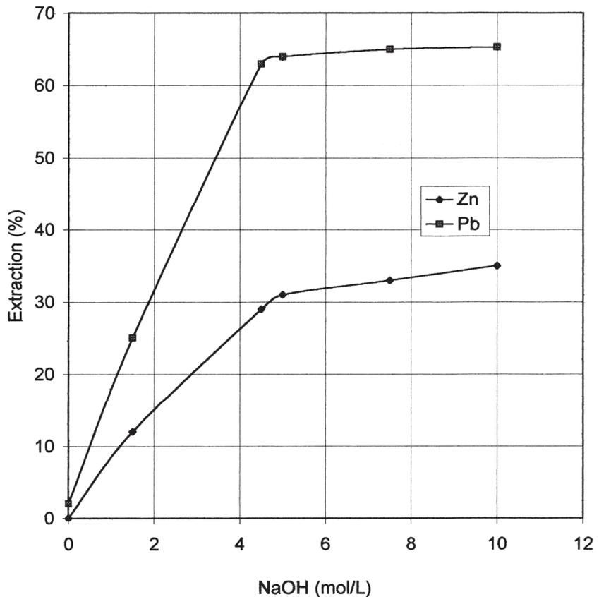
**Figure 17.** Effect of NaOH concentration on the extraction of Zn and Pb from steelmaking dust (25 °C, L/S 3.6, leaching time 42h) [7].
