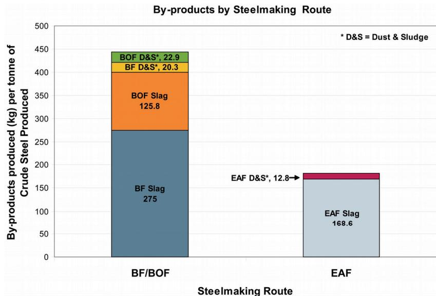
**Figure 2.** By-products formed in steelmaking routes [12].
