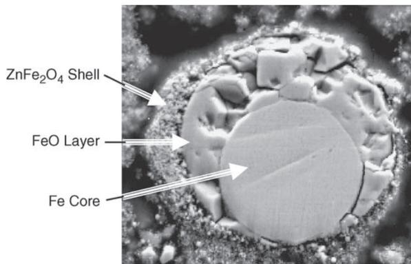
**Figure 3.** A spherical particle from BOF sludge [17].
