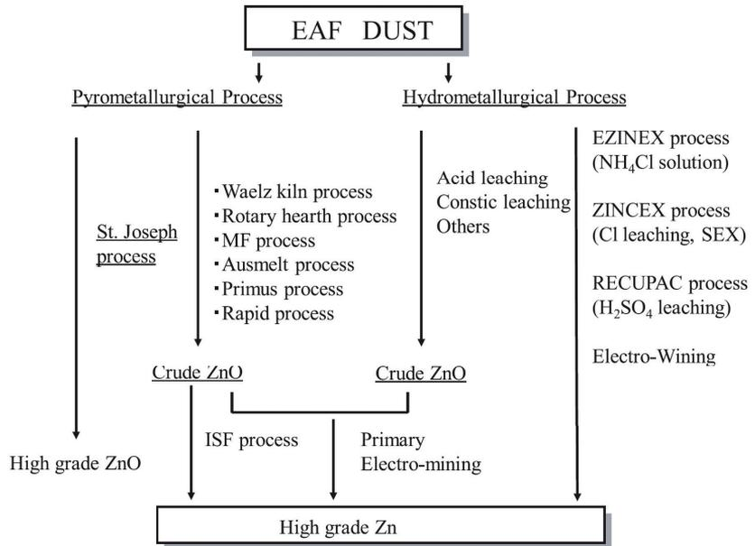
**Figure 8.** Pyro- and hydrometallurgical treatment processes of EAF dust [26].
