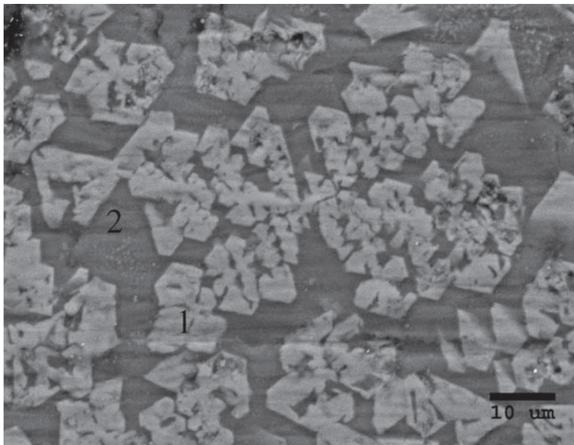
**Figure 7.** Dendritic structure in a EAFD particle (area 1: rich in Fe, Cr and O, area 2: rich in Fe, Ca, Si and O) [25].
