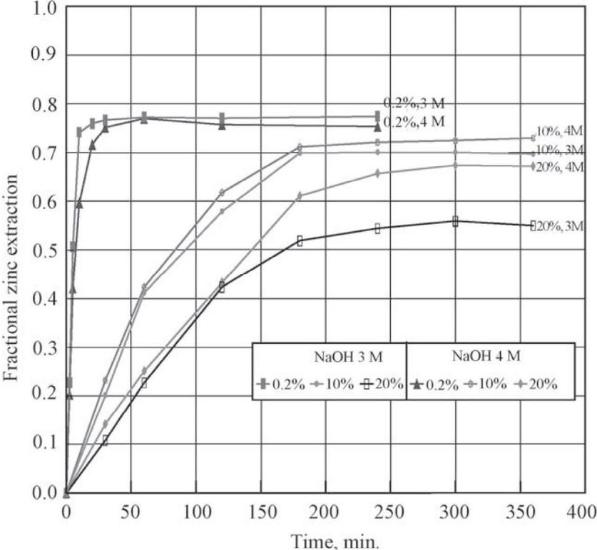
Figure 19. Effect of solid content on leaching rate (850 rpm, 95 °C) [35].
