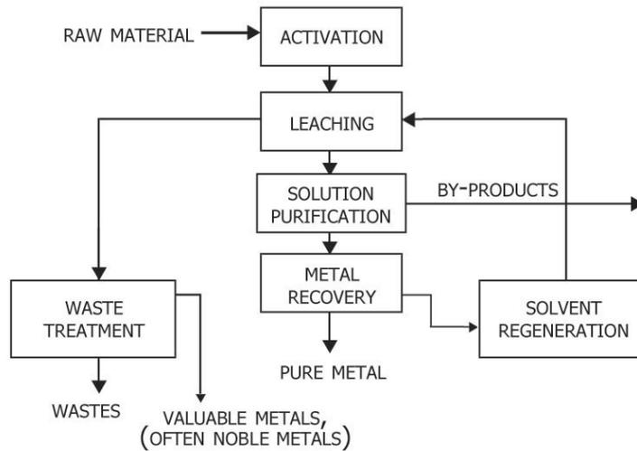
**Figure 11.** The common stages in a hydrometallurgical process.
