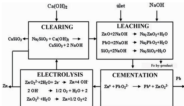
Figure 12. Principle of the Cebedeau-process [53].
