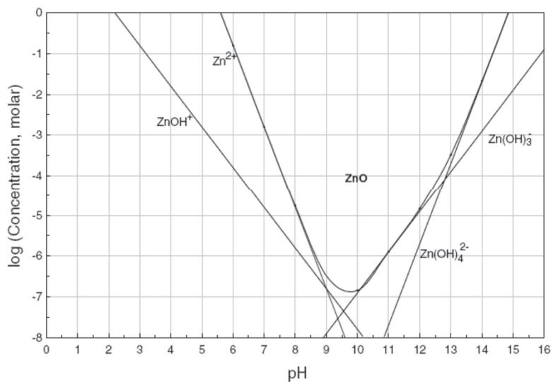
**Figure 15.** Solubility of ZnO as a function of pH, at 25 °C [14].
