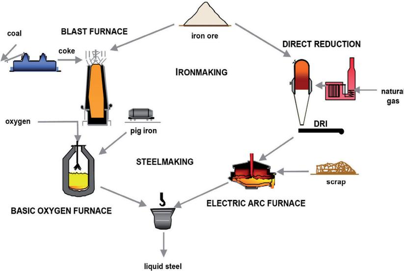
Figure 1. Steelmaking routes [10].
