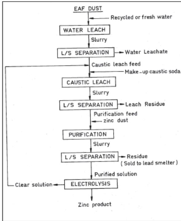
**Figure 14.** A principal flowsheet of caustic leach-electrolysis process [30].
