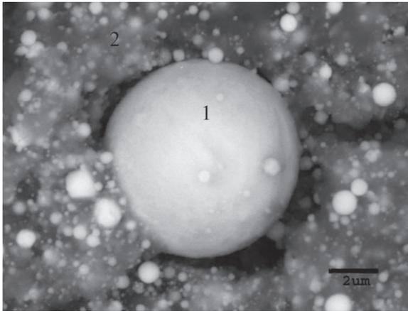
**Figure 6.** A spherical EAFD particle (area 1: rich in Fe and O, area 2: rich in Fe and Zn) [25].
