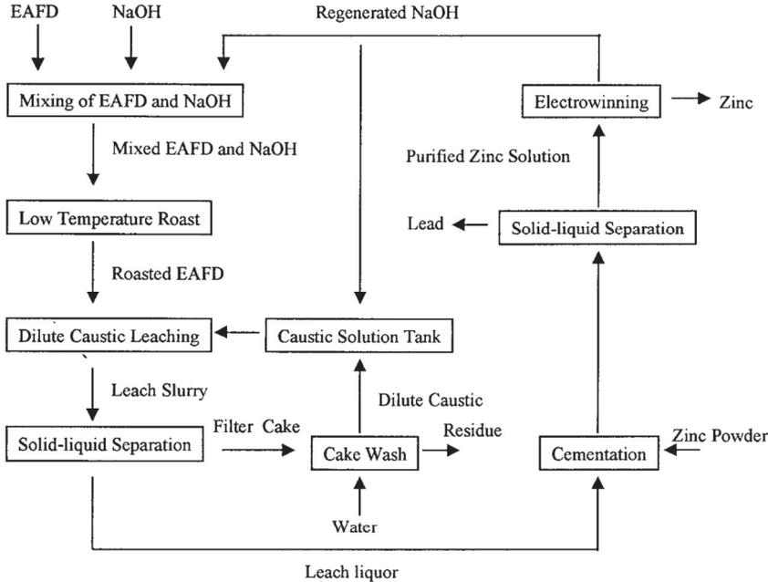
**Figure 20.** Flowsheet of caustic soda roasting and leaching treatment process for EAFD [5].
