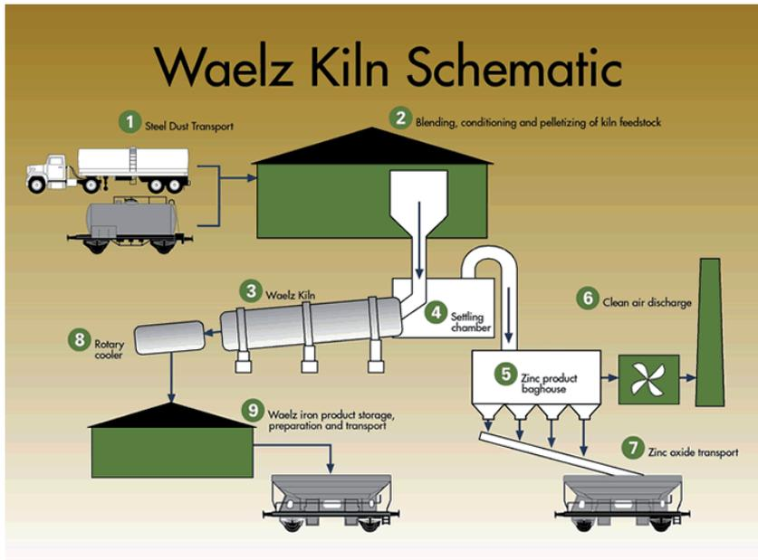
**Figure 9.** A schematic presentation of dust recycling route via Waelz Kiln [44].
